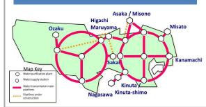
A network of water transmission pipes extending throughout Tokyo ensures backup functionality in the event of accidents or natural disasters.
