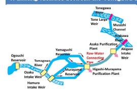
Raw-water connecting pipelines 2200mm in diameter link between separate rivers, allowing water to be received from either source.
