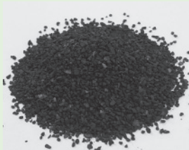
Granular activated carbon used for advanced water treatment
