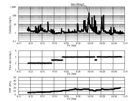
Figure 3 - Changes of turbidity in the source water, flow rate and TMP during the plant-scale experiment
