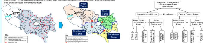
Figure 2 - Distribution of central control rooms and facilities (1984) Figure 3 - Distribution of central control rooms and facilities (2008 to present) Figure 4 - Hierarchical Structure of Tama Monitoring Control System
