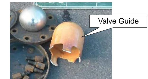
Pictures 3 and 4. Damage to a quick air-valve in the Tohoku Region
