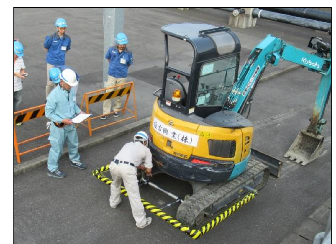
Figure 7: Reoccurrence prevention measures shared among contractors (equipment to stop backhoe collisions)
