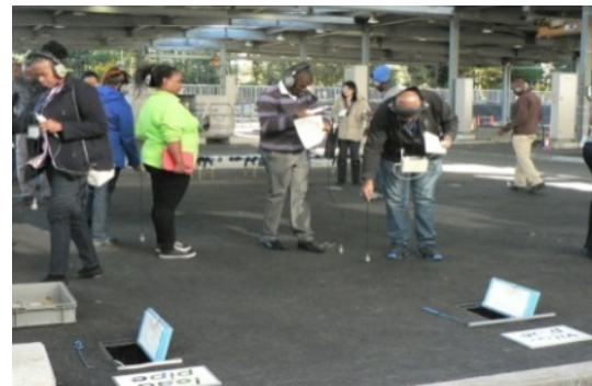
Figure 3.2 Leakage Detection (At the Training and Technical Development Centre, Bureau of Waterworks, Tokyo Metropolitan Government)
