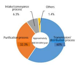
Fig. 1 Breakdown of electric power consumption
