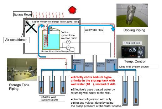
Fig. 9 Sodium Hypochlorite Storage Tank Cooling Flow
