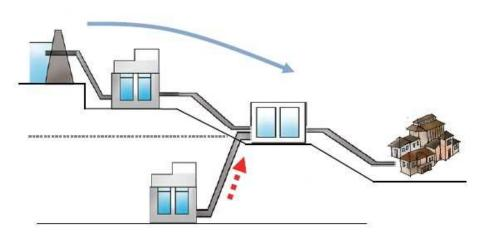
Figure 7: Water transmission utilizing gravity flows
