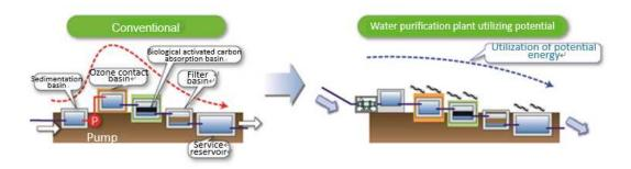
Figure 5: Water purification plant utilizing potential energy
