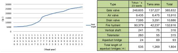
Figure 1: Total extension of managed pipelines in Tokyo by fiscal year
