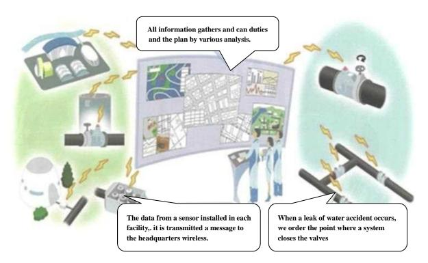
Figure 9: Effect by the total management system Source of reference : [Pipe Stars Project] Published by Japan Water Research Center
