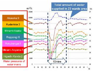
Figure 11 Changes of water supply and water pressure during the Kumamoto earthquake
