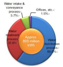
Figure 2 Breakdown of electricity usage
