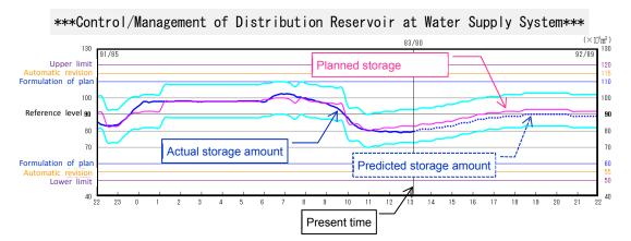
Figure 5 Prediction and Actual Record in Distribution Reservoir Operation System
