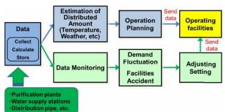
Figure 4 Roles of the Water Supply Operation Center
