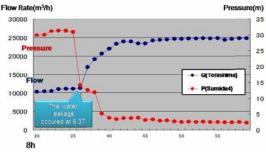
Figure 7 Changes in flow rate and pressure during an accident
