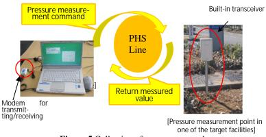
Figure 5 Collection of water pressure data
