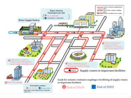
Figure 2 Seismic resistant coupling retrofitting of supply routes to important facilities (conceptual diagram)
