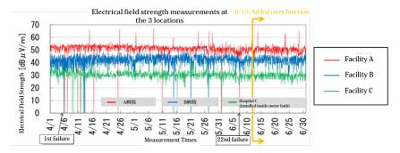
Figure 11 Communication test and electrical field strength
