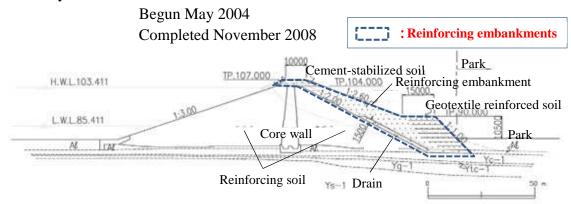
**Fig. 12**: Cross-sectional diagram of the Lower-Murayama Reservoir dam body reinforcements
