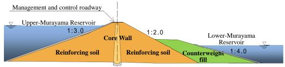
Fig. 14: Upper-Murayama Reservoir, existing dam body – Standard cross-sectional diagram
