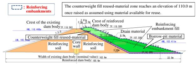
Fig. 15: Reinforced dam body – Standard cross-sectional diagram
