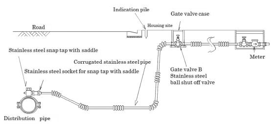
Figure 1 Water supply equipment to be buried beneath the roads
