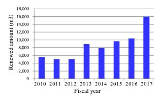
Figure 2: Amounts of granular activated carbon renewal
