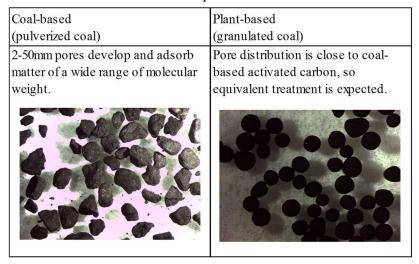
Furthermore, unlike coal-based activated carbon, plant-based activated carbon has no risk of elution of heavy metals such as arsenic, and also as coconut shell, its raw material, is a non-depleting resource, it is possible to produce consecutively, and risk reduction at time of procurement is possible by using in combination with a coal-type. These are some of the many merits attributed to the introduction of plant-based activated carbon.
