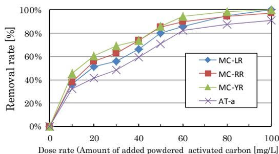
**Figure 3** Removal of MCs and AT-a by powdered activated carbon (Experiment No. 1)
