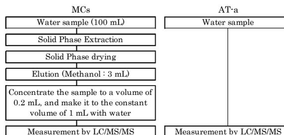
**Figure 1** Analysis procedure of MCs and of AT-a
