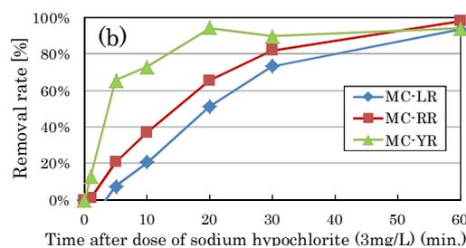
**Figure 4** (a) Removal of MCs and AT-a by sodium hypochlorite (Add MCs and AT-a to ultrapure water (Experiment No. 2) ; (b) Add MCs to raw water in Ozaku purification plant (Experiment No. 3))
