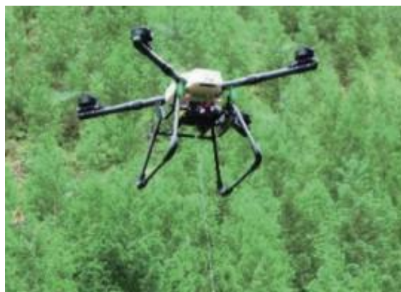
Drone transporting materials for protective fencing
