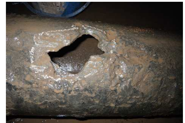
Fig.2 Corrosion leakage of iron pipes
