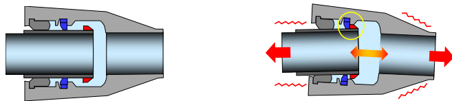
Fig.8 Earthquake-resistant joints... Structure that does not cause joint detachment during the earthquake (Left: Normal Condition, Right: Earthquake Condition) 4
