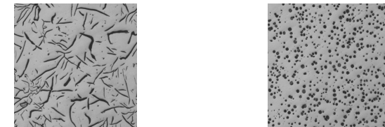
Fig.9 Micrograph of cast iron (Left: High-grade cast iron, Right: Ductile cast iron)
