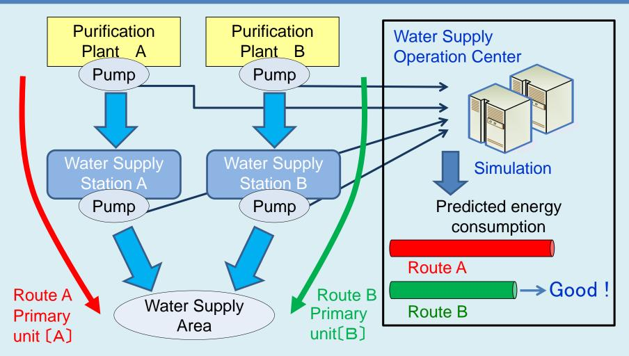
Primary unit of distributed water (kWh/m<sup>3</sup>) × Flow rate Q(m<sup>3</sup>) = Predicted energy consumption (kWh)
