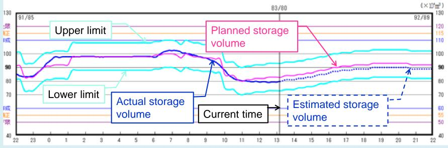
Time fluctuation of storage volume at distribution reservoirs
