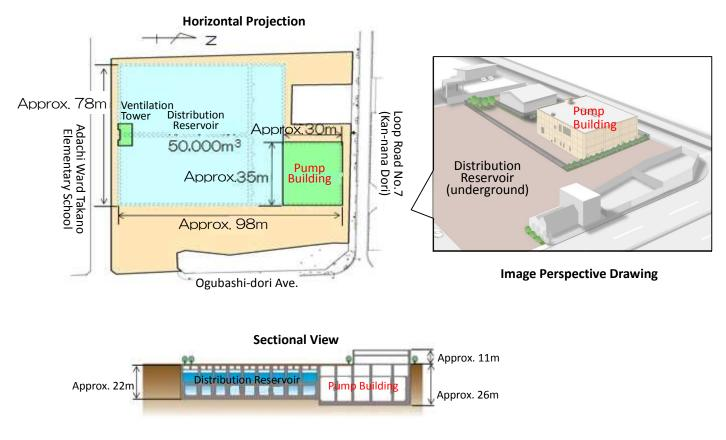
Figure 5: Layout of Kohoku Water Supply Station
