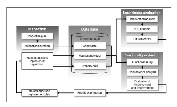
Figure 3: Conceptual Diagram of Asset Management
