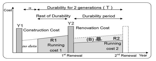
Figure 4: Image of Calculation of Life Cycle Cost
