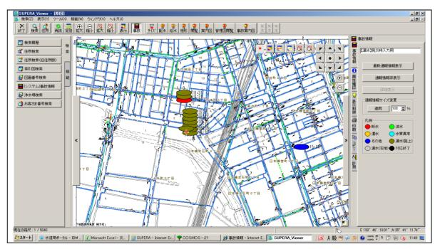
Fig. 4: Displaying leakage information in the GIS database
