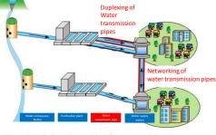
Figure 4 Duplexing and networking of water transmission pipes
