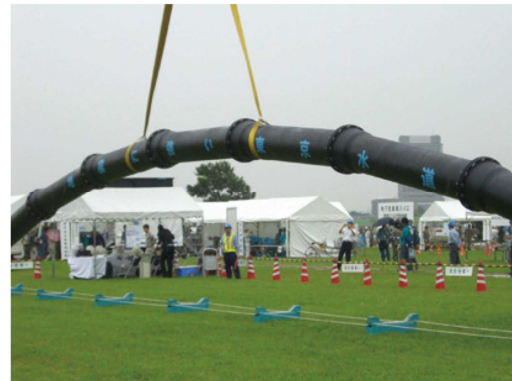
Photo 2: Demonstration of Earthquake-resistant Joint Pipes
