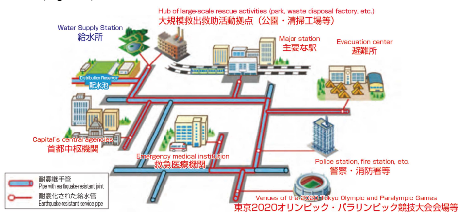
Figure 6: Pipe Jointing by Earthquake-resistant Joints in Water Supply Pipes Connected to Important Facilities
