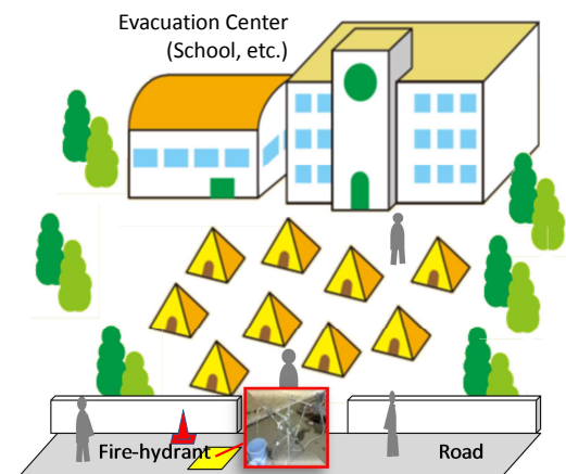
Figure 5: Image of Emergency Water Supply from Fire Hydrant around Evacuation Center
