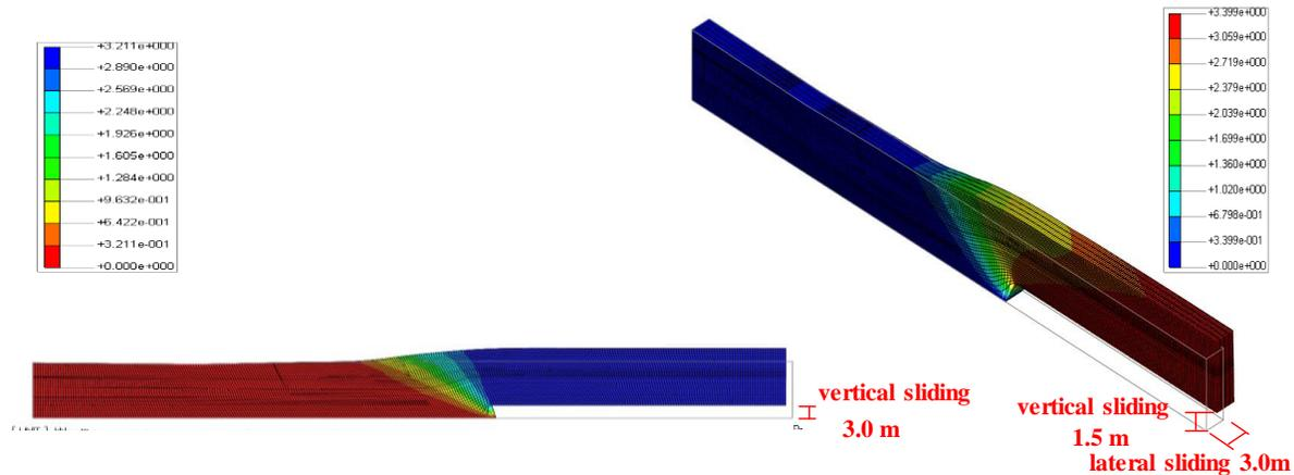
Figure 7: Fault Displacement Contours
