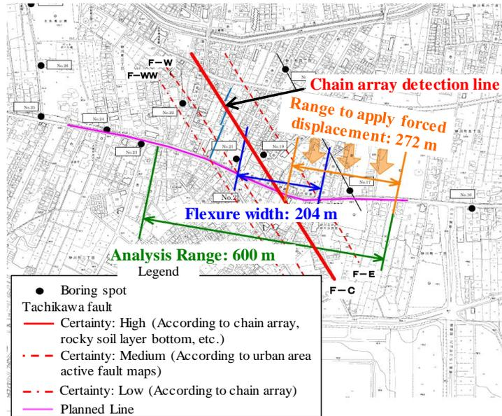
Figure 5: Analysis range to calculate ground deformation caused by faults
