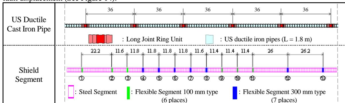
Figure 14: Arrangement of US ductile cast iron pipes and shield segments
