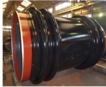
Figure 9: Steel pipes for faults
