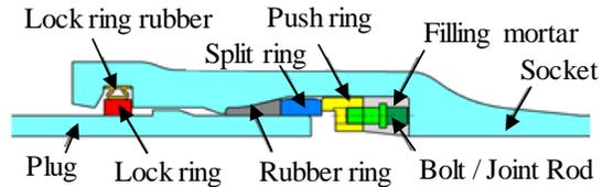
Figure 12: US Ductile Cast Iron Pipe
