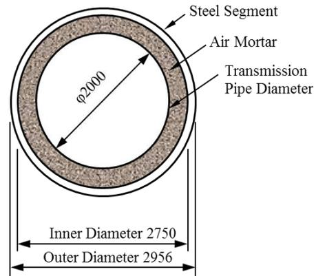
Figure 3: Standard Cross Section
