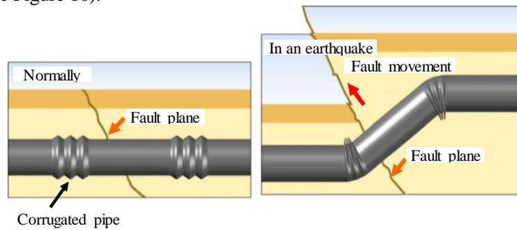
Figure 10: Fault displacement mechanism
