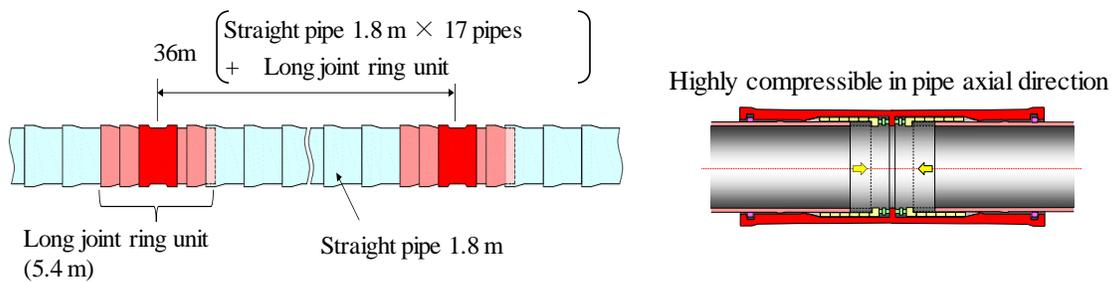
Figure 13: Major displacement pipeline system with long joint ring units
