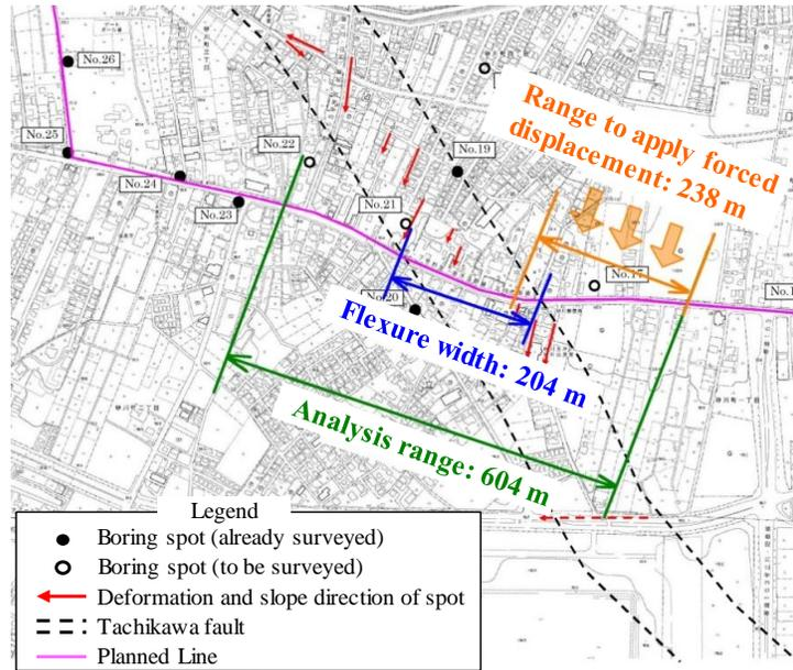
Figure 4: Range in which to analyze ground deformation
