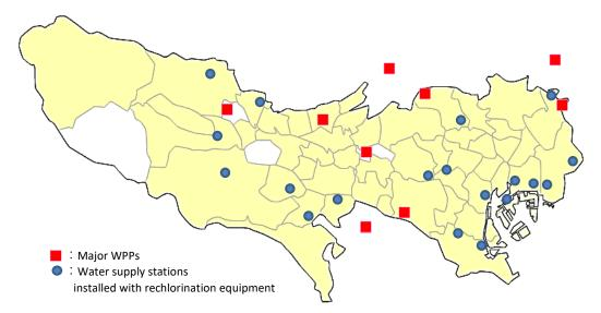
Figure 4 Sites where additional chlorine injection facilities are installed
