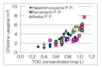
Figure 6 Relation between TOC concentration and chlorine usage
