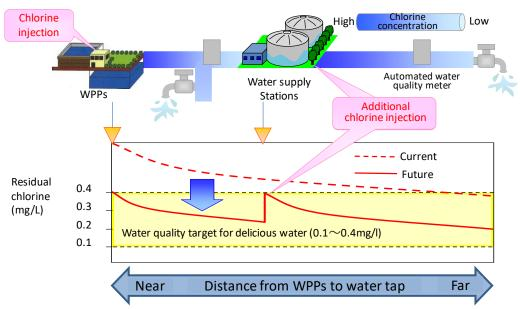
Figure 3 The effect of additional chlorine injection facilities
