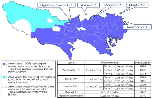
Figure 2 WPPs with advanced water treatment installed and their capacity
