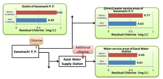
**Figure 8** Change of residual chlorine concentration before and after additional chlorine injection in the water supply district of Kanamachi P. P.
