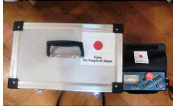
▲ Electronic leakage detector made in Japan
