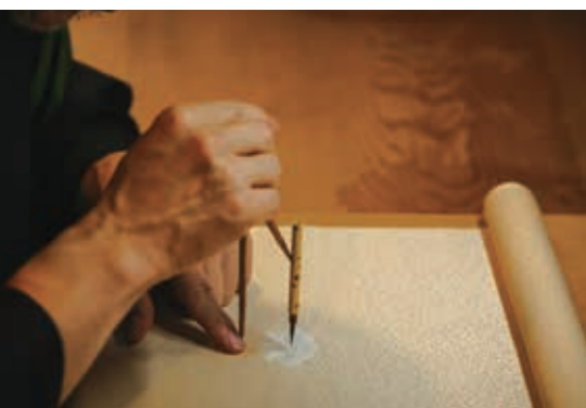
The bun-mawashi (bamboo compass) has been used for centuries in the design of kamon .
