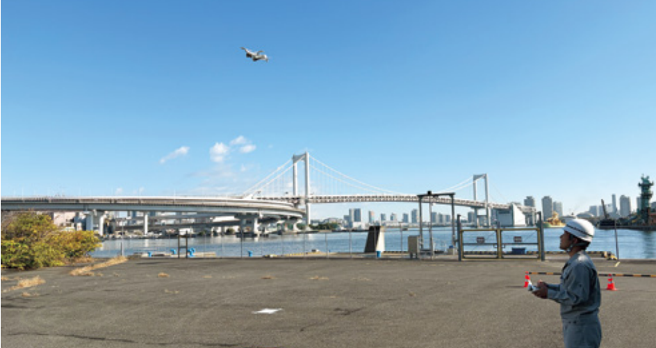
A beyond-visual-line-of-sight flight test is being conducted, with drones inspecting coastal protection facilities over a wide area.
