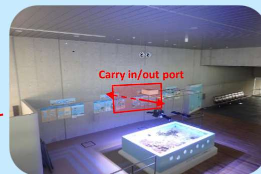
To renew the equipment inside the machinery room, it must pass through the viewing route, making it necessary to close the viewing area each time.
