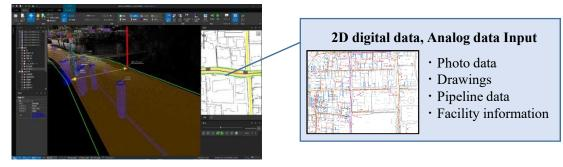
• 3D representation of underground facilities such as water pipes makes it possible to understand the status of underground facilities in 3D, rather than simple lines and surfaces.
